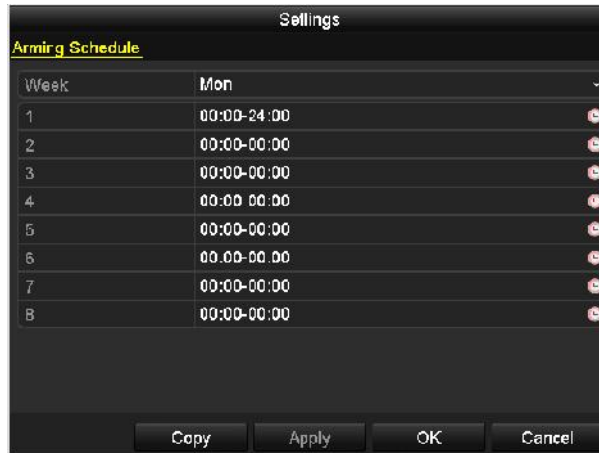
Figure 8. 20 Set Arming Schedule of Alarm Output
